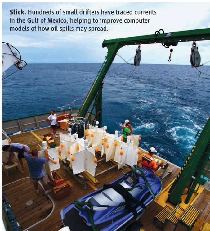
**Slick.** Hundreds of small drifters have traced currents in the Gulf of Mexico, helping to improve computer models of how oil spills may spread.
